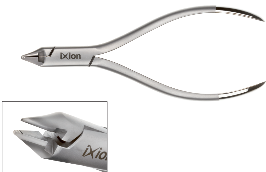
ix808 Light Wire Plier with Cutter and 2 Grooves The most popular wire bending plier. The Inserted tips provide excellent wear and bend archwires from .012" to .020" (.30mm - .51mm). Beaks are grooved for round wire at 1mm and 2mm from tip. Cutter at the base of beaks cuts archwires from .014" to .020" (.36mm - .51mm).
