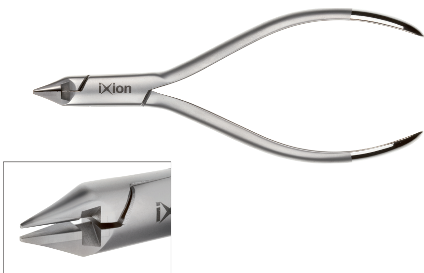
ix809 Light Wire Plier with Cutter This popular loop forming and bending plier. Has inserted tips that provide excellent wear. The precise round and square tips bend archwires from .012" to .020" (.30mm - .51mm). Cutter at base of beaks cuts archwires from .014" to .020" (.36mm - .51mm).
