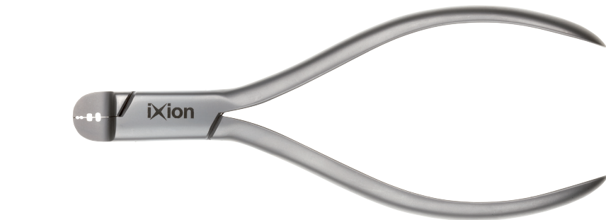
ix705 Lingual Arch Bending Plier Grooved to hold all larger wire sizes, jaw width is .120" (3.05mm). Also ideal for double and triple back bends. Bends round, square and rectangular wires up to .036" (0.91mm) max.
